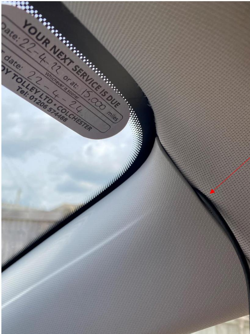
Run the cable around the head liner to the driver's door front pillar. It slides in quite easily with the use of come trim tools.
