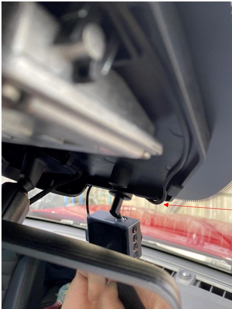
Prise off the above mirror cover and route the cable from the dash cam into the void.
