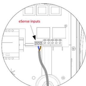
Connect the eSense cables using the diagram
