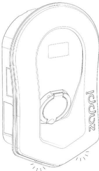
Ensure the 2 tabs at the bottom of the fascia click to indicate its securely fixed in place.
