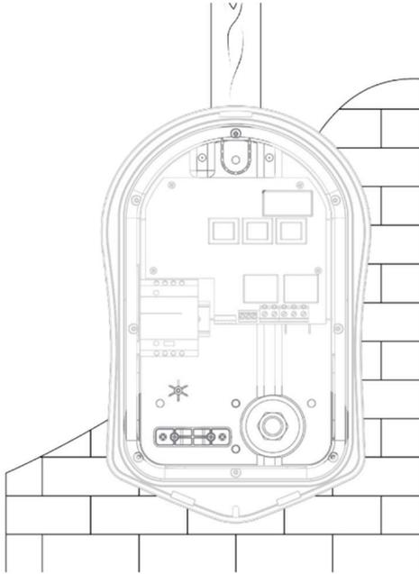
Using **zappi** template mark mounting holes. For fixing to brick, use the top and 2 bottom holes (left/right). Use the 2 vertical holes as well as the top hole if mounting to a stud wall or joist.
