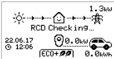
zappi is carrying out a check to make sure that the built in RCD and "PEN Fault" protection is working before starting to charge the car. zappi carries out this before every charge so there is no need to manually test the RCD protection.
