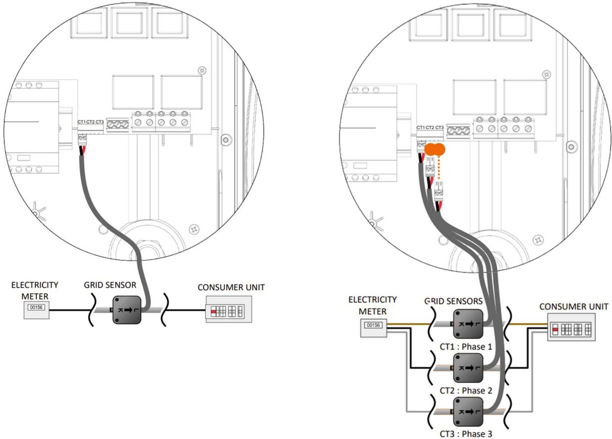
**SINGLE PHASE:** A CT clamp must be placed around the live meter tail as shown above with the arrow pointing towards the consumer unit
