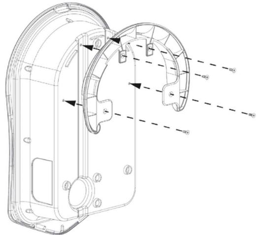
If installing a tethered zappi, you must ensure the cable wall guard is fixed to the unit using the 4 screws supplied.
