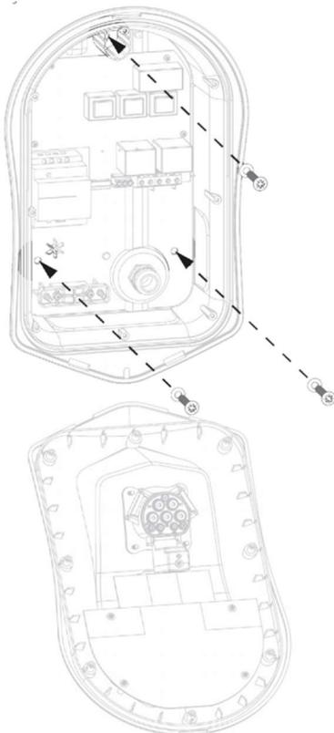
Secure the unit to the wall using the fixing kit provided. Ensure the grommets are used to maintain its IP integrity.
